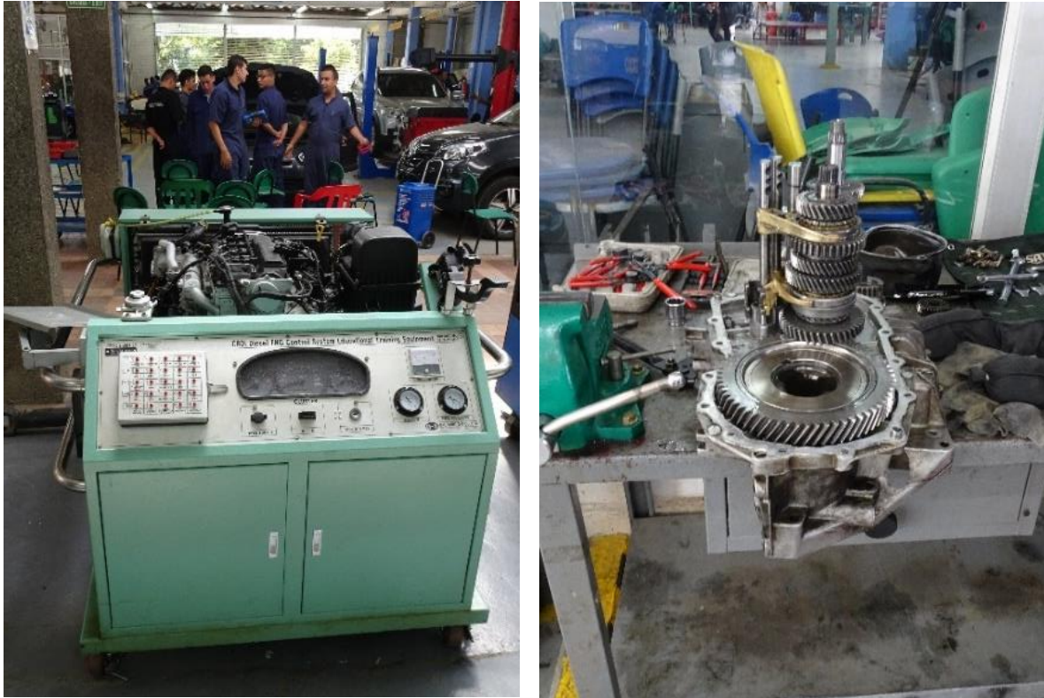
Image 8: dismantled gearbox and modified engine for education purposes.
