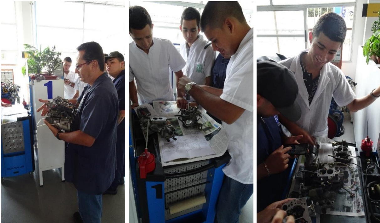
Image 16: a teacher at the Institución Universitaria Pascual Bravo explaining the functions of a carburetor and students disassembling and assembling different models of carburetors.
