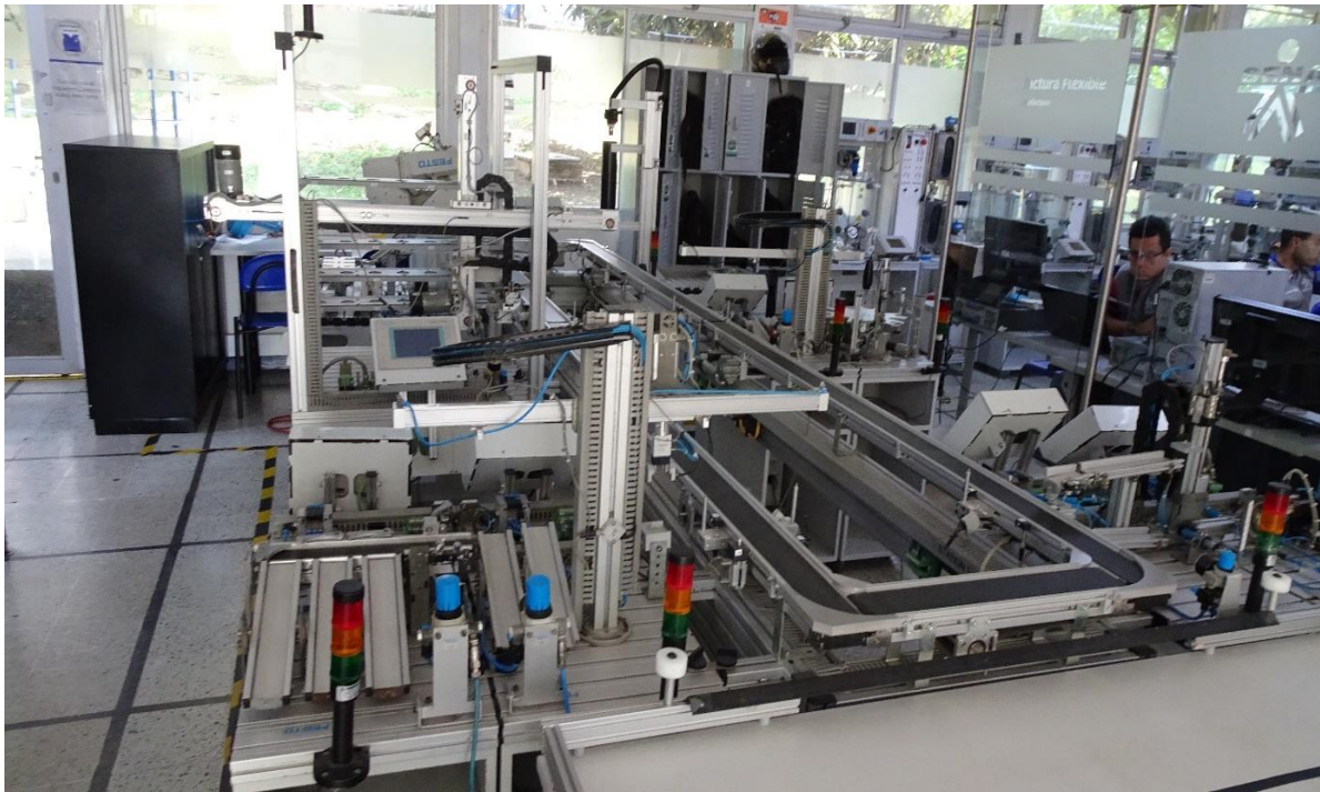
Image 12: fully functioning model of automatized production line.
