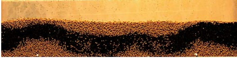
(a) Experiment 10.1, radial segregation at low fill level and slow rotation speed.
