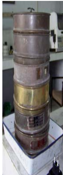
Figure 21: The machine made by Prashant Vipul to sieve out the granulate 62 .
