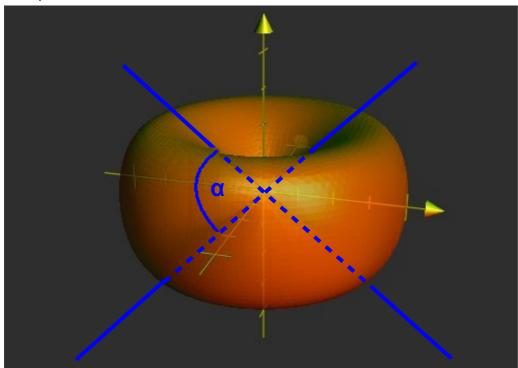
The outer surface area of the ring is about:  $\alpha/180^{\circ}$  x  $(4 \pi r^{2})$  = 1/1.64  $(4 \pi r^{2})$  for dipole antennas.
